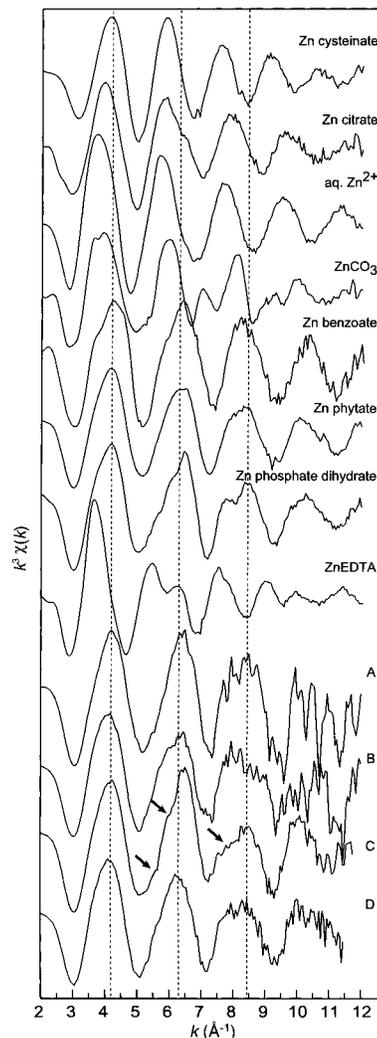
FIGURE 2. Comparison of Zn K-edge EXAFS spectra for *P. vulgaris* grown in ZnEDTA- (A: roots, B: leaves) and Zn sulfate- (C: roots, D: leaves) containing nutrient solution and for a selection of model compounds. The sample "aq. Zn<sup>2+</sup>" corresponds to a solution containing 0.1 mol/L Zn(NO<sub>3</sub>)<sub>2</sub> at pH 4, whose calculated Zn speciation is 100% Zn<sup>2+</sup>.
